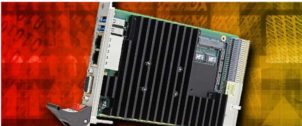
Equipped with Intel's latest Atom processor Apollo Lake-I, the low-power CPCI PlusIO board F26L has a total power consumption of max. 6.5 to 12 W, while providing a 1.6 GHz clock frequency, excellent graphics performance, board supervision features, TPM and Intel VT virtualization technology.
