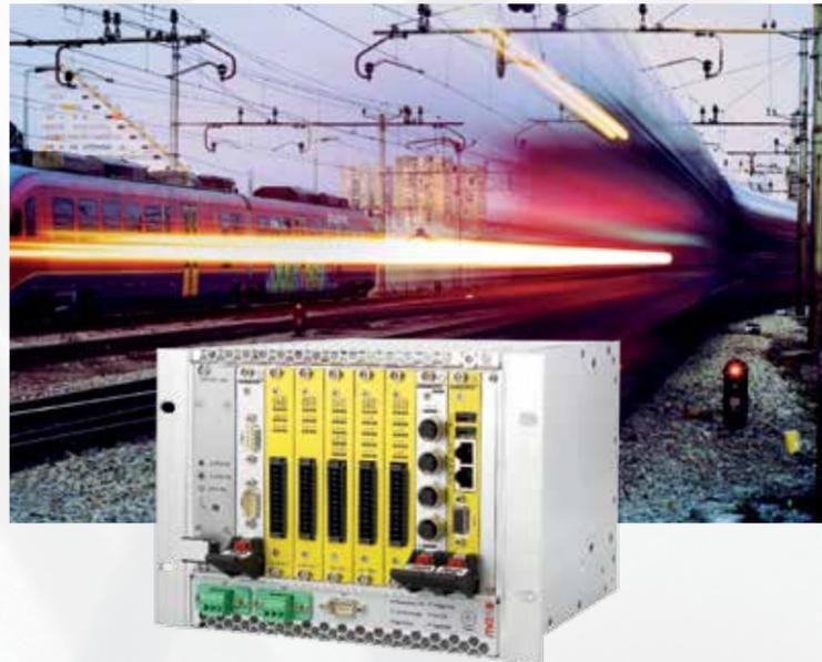
The MH50C is the central controller of the MEN Train Control System and is a modular system platform usable for safety-critical train applications like train control, automatic train operation (ATO) and automatic train protection (ATP).
