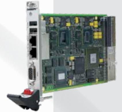
The CompactPCI PlusIO SBC unites three CPUs on one 3U CompactPCI® PlusIO card. It makes Intel® Atom™ E6xx (“E600”) performance with dual redundancy extremely compact and can replace multiprocessing systems by a flexible small-footprint, low-power solution.
